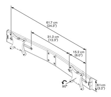
The two monitors will be perfectly aligned next to each other and move as one monitor. PFA 9102 is available for mounting two monitors vertically above each other. This mount supports up to 6.5 kg for each monitor. PFA 9102 fits the PFD 8522, 8523, 8541 and 8543.
