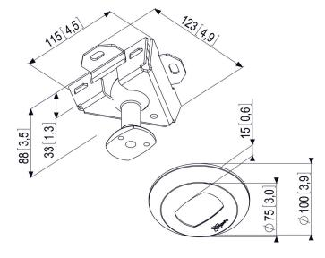
This ceiling plate is suitable for flat and inclined ceilings. The screen can be turned in any required position by using the ball joint in the ceiling plate. Combine this ceiling plate with one of the poles from the Connect-it Series (PUC 2108, PUC 2115, PUC 2130, PUC 2308, PUC 2315 or PUC 2330) and a Connect-it interface (PFI 3010, PFI 3020, PFI 3030 or PFI 3040) for a complete ceiling solution.
