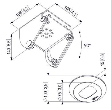
This ceiling plate is suitable for flat and inclined ceilings (up to 90°). Combine this ceiling plate with one of the poles from the Connect-it Series (PUC 2108, PUC 2115, PUC 2130, PUC 2308, PUC 2315 or PUC 2330) and a Connect-it interface (PFI 3010, PFI 3020, PFI 3030 or PFI 3040) for a complete ceiling solution.
