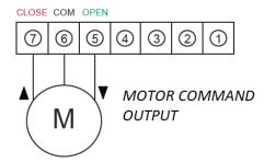
MOTOR OUTPUT CONNECTION: connect the cable OPEN of the motor to the clamp 5 (motor wire brown), the cable CLOSE to the clamp 7 (motor wire black) and the COMMON motor cable to the clamp 6 (motor wire blue). Motor wire yellow/green will not be connected.
