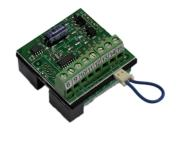
Control unit for one electromechanical motor, centralization or integration dry contact command.
